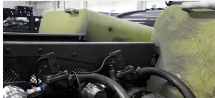
Air amplifiers for profiles' cleaning
