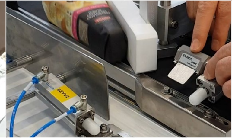
Air knife for defective parts' discard
