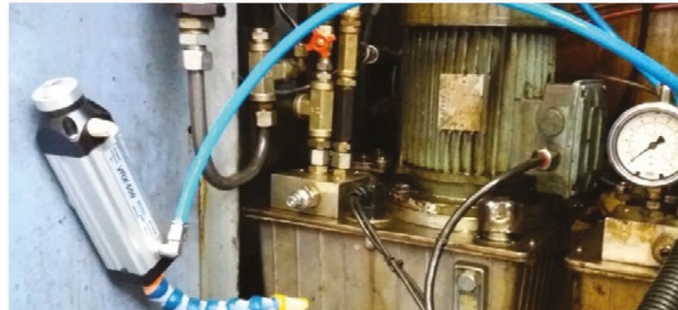
Cooler for hydraulic application
