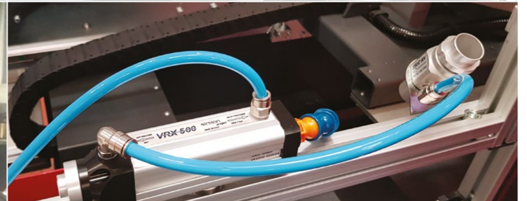
Cooler for making window fixtures
