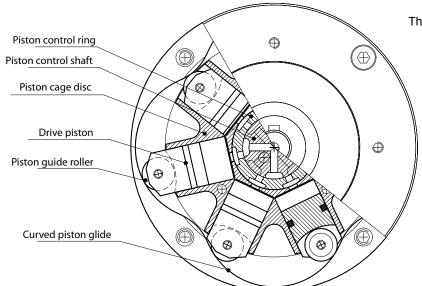
The rollers of the cylinders are fabricated of high stress plastic material and run on double bearings. This allows for low friction with minimal noise and high life expectancy. Compared to standard air motors these pneumatic motors model EasyDrive have their highest torque rating at low revolutions and minimal air consumption.
