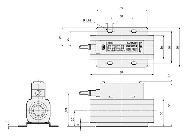
Display separated, port size: push-in φ4, φ6, Rc1/8, M5
