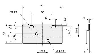
\* 2 M3 fixing screws (length 6 mm) attached
