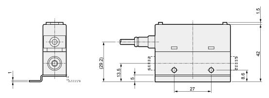
Display integrated, port size: push-in  $\phi 8$ ,  $\phi 10$ , Rc1/4
