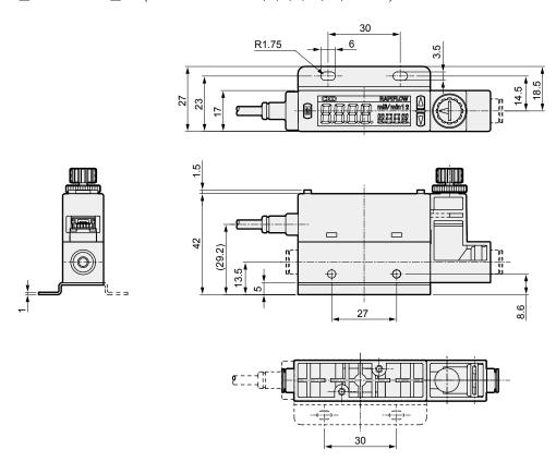
Needle valve integrated, port size: push-in φ8, φ10, Rc1/4
