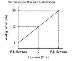
With the display integrated bi-directional, output can be changed to uni-direction output with the button settings. Refer to page 1278 for details.
