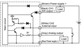
$^*$  Analog output: Voltage output R: approx. 1 k $\Omega$  Current output R: approx. 100  $\Omega$
