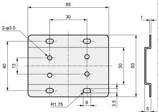
\* 2 M3 fixing screws (length 6 mm) attached
