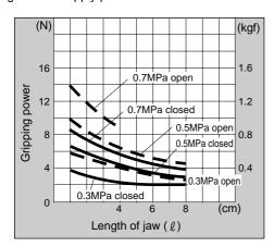
■ To obtain gripping power from performance data, if the distance to the workpiece's center of gravity is \( \ell \) when manufacturing the small jaw, gripping power F is expressed as follows
