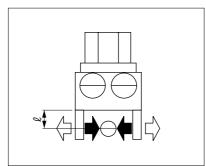
Performance data indicates the gripping power at hand jaw length \( \ell \) at a supply pressure of 0.15 to 0.7 MPa.
