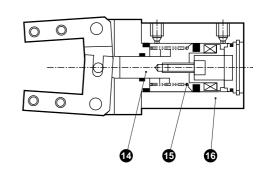
\* Spring of **(** is not contained in standard (double acting) type.
