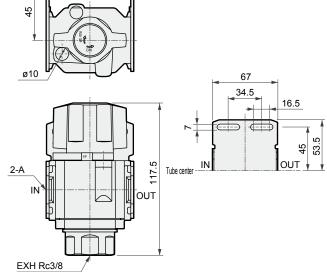
The C type bracket is attached at shipment. C type bracket and piping adapter set can not be used together.
