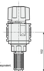
Silencer will not be installed upon shipment. Silencer is flame resistant resin UL94 standard V-0 equivalent. However, element is not flame resistant.
