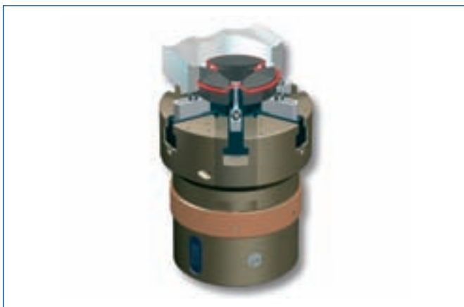
3. Travel into the bore (assembly position) and pressing by triple jaw B.
