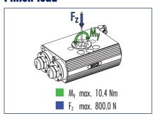
Moments and forces may occur simultaneously. When using heavy attachments or ones with high mass moments of inertia, the speed must be restricted to ensure that the rotary movement occurs without any hitting or bouncing.
