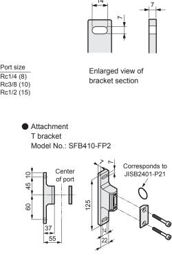
Material: Aluminum die-casting Mounting screw with stainless steel
