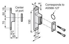
Material: Aluminum die-casting Mounting screw with stainless steel
