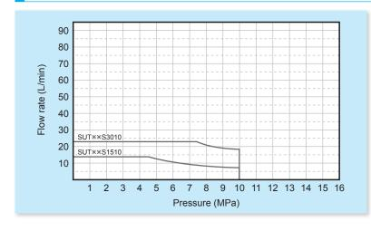
\* Operating flow rate at the maximum pressure in continuous operation: SUT \*\* \$1510: 3 L/min maximum SUT \*\* \$3010: 5 L/min maximum
