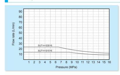
\* Operating flow rate at the maximum pressure in continuous operation: SUT \*\* \$1516: 5 L/min maximum SUT \*\* \$3016: 5 L/min maximum
