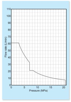
$^{\star}$  Operating flow rate at the maximum pressure in continuous operation: 6.5 L/min maximum
