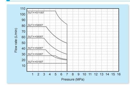
\* Operating flow rate at the maximum pressure in continuous operation: SUT \*\* \$1507: 3 L/min maximum SUT \*\* \$3007: 5 L/min maximum SUT \*\* \$4007: 8 L/min maximum SUT ×× S6007: 14 L/min maximum SUT \*\* \$8007: 19 L/min maximum SUT\*\*S11007: 16 L/min maximum
