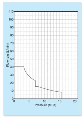
\* Operating flow rate at the maximum pressure in continuous operation: 8 L/min maximum
