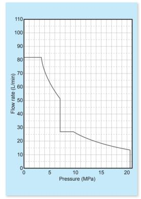
\* Operating flow rate at the maximum pressure in continuous operation: 14 L/min maximum
