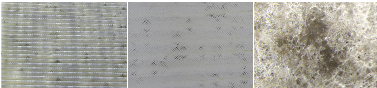
Filter materials with discharge traces when using zinc and ash-free oil.
