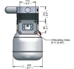
Allow 180 mm (7") below pump for Reservoir removal.
