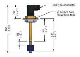
Note: Dimensions shown are for the T10 Stem length for T30 is 50mm longer
