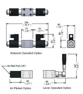
W2 Series ultra low leakage Poppet Directional Valves -CETOP03/DO3/NG6 manifold interface.
