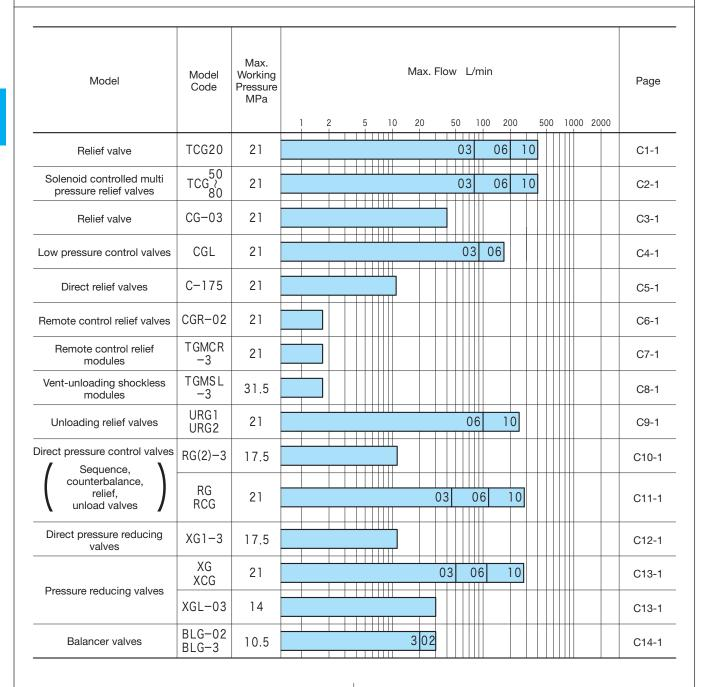
Pressure control valves are used to limit pump delivery pressure, control circuit pressure, and as safety valves. For these purposes there are relief valves and reducing pressure valves which maintain circuit pressure below set levels, and sequence and unload valves which automatically switch circuits when circuit pressure reaches setting pressure.
