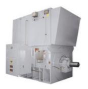
Pressurized - Ex p (EPL Gb or Gc): type of protection in which the equipment is manufactured to operate with positive internal pressure so as to avoid the ingress of flammable gases and vapours into the enclosure, where there are parts which may cause the ignition of an explosive atmosphere. Standard: IEC 60079-2 - Explosive Atmospheres - Part 2: Equipment Protection by Pressurized Enclosures "p".
