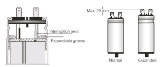
Fig. 1 Internal view of UCWs
