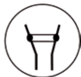
IEC/EN 60947-5-1 Mechanically linked contacts
