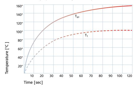
The maximum temperature must not exceed the manufacturer's maximum permitted temperature for the friction material, otherwise the linings may be damaged. This can lead to a loss of effectiveness of the brake and, in the worst case, destruction of the brake.
