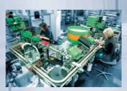
Assembly and testing of pressure switches on partially or fully automated plant.
