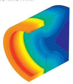
The temperature distribution illustrated above on a sectioned brake drum clearly shows the higher heating of the drum in the region over the flyweights.
