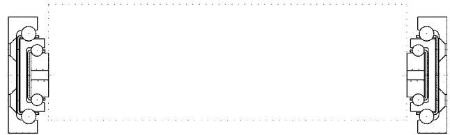
Standard application: Drawer extension telescopic rails vertical.
