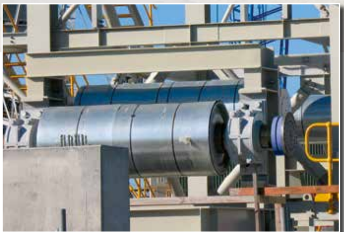
Belt drum with Locking Assemblies and a shrink disc on the drive side
