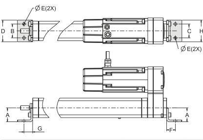
The foot mount consists of a front and rear bracket and comes mounted from the factory if the ordering code states that the unit shall be equipped with one. It can also be ordered as a separate part (all necessary actuator attachment screws are included) using the part number.
