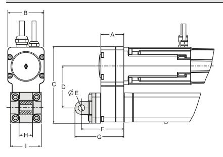
The rear clevis consists of a bracket and comes mounted from the factory if the ordering code states that the unit shall be equipped with one. It can also be ordered as a separate part (all necessary actuator attachment screws are included) using the part number.
