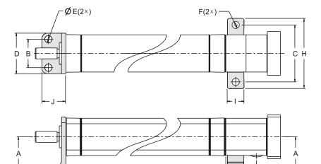
The foot mount consists of a front and rear bracket and comes mounted from the factory if the ordering code states that the unit shall be equipped with one. It can also be ordered as a separate part (all necessary actuator attachment screws are included) using the part number.
