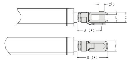
The front clevis comes mounted from the factory if the ordering code states that the unit shall be equipped with one, but it can also be ordered as a separate part using the part number. To be able to mount a separate front clevis the extension tube must be equipped with a male threaded rod end.
