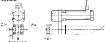
The fixed front and rear trunnions consist of a plate with two shafts and come mounted from the factory if the ordering code states that the unit shall be equipped with one. They can also be ordered as a separate parts (all necessary actuator attachment screws are included) using the part numbers. The rear trunnion can only be mounted on to the belt gear on parallel style actuators.
