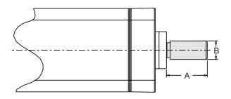
The male threaded rod end comes mounted from the factory if the ordering code states that the unit shall be equipped with one.
