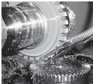
CNC machining of a PowerTRUE™ right angle gear
