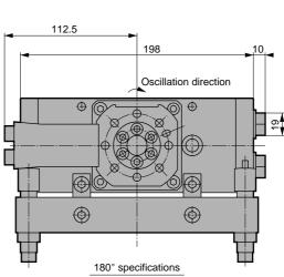
Note: Dimensions of rotary actuator main body are as same as basic type, however the body can not be fixed with using 4 taps on main body top. Position for dowel hole differs depending on installation position of outer mount shock absorber on table top. (Refer to GRC-5-\*-A1/A2.)
