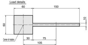
(Distance from center of rotation to rectangle plate load center)
