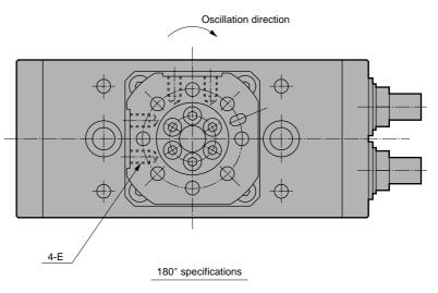
When outer mount shock absorber set is installed. ([ ]](shaded section) shows outer mount shock absorber set.) Note: When outer mount shock absorber set is installed on A3 type, A1 type is provided. Consult with CKD on A2 type. (Refer to Page 34 for installation position.)
