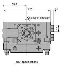
Note: Dimensions of rotary actuator main body are as same as basic type, however the body can not be fixed with using 4 taps on main body top. Position for dowel hole differs depending on installation position of outer mount shock absorber on table top. (Refer to GRC-5-\*-A1/A2.)
