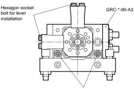
External shock absorber hexagon socket head cap bolt for installation
